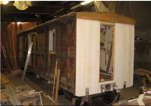
Here we see some of the car's new siding being installed. However, as the original siding was being removed, we discovered an end door that was covered over during a past rebuild decades ago. Since we are returning this car to its 1930's configuration, this end door will be reinsulated.
